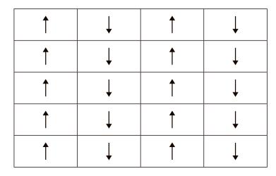
When installing this product, as indicated in the figure above, place the row of up-facing and the row of down-facing alternately.
